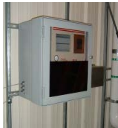
Model 301C (Above) mounted downstream of a waste incinerator measuring H_2S & CH_3SH at ppb levels via PID.
