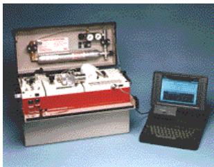
Portable GC for On-Site Measurements of 1,3 BD
