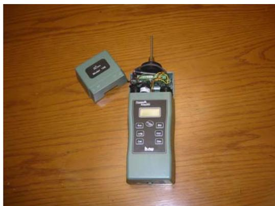
**Fig.2. PID-106 Analyzer with 3 gas sensors and the MICA2+MDA320 module installed.**
