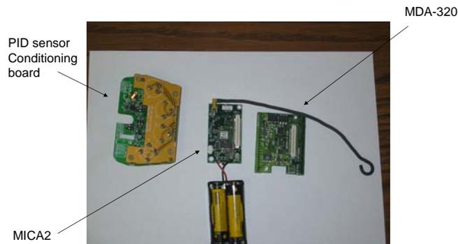
Fig.1. PID sensor board, MICA2 radio, and MDA320 8-channel 16-bit resolution Analog to Digital Conversion board.
