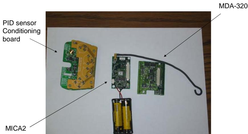
**Fig.3. Elements of the Mesh Network: the computer with the base mote, PID-106 with MICA2+MDA320 module installed, and the MICA2+GPS module.**
