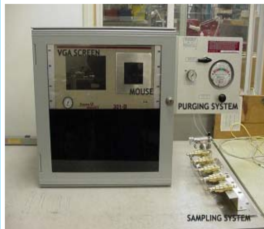
Explosion proof (Z purge) 301C (above) with external air activated multi (5) point system with moisture removal.
