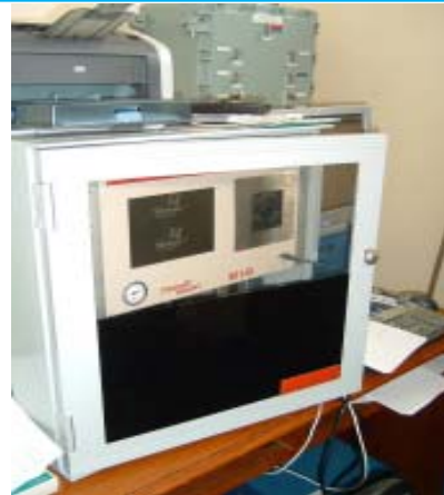
301C installed at a natural gas odorant facility for measuring THT & TBM on-line.
